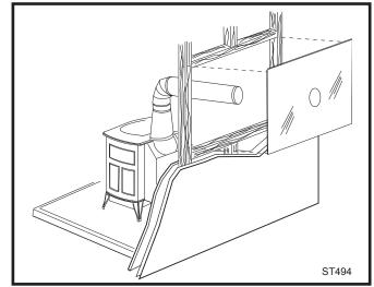
Fig. 9 A hollow wall pass-through method.
